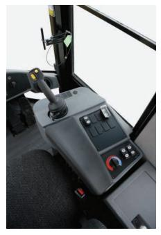
**VISIBILITY.** The 938H offers excellent visibility to the front and rear of the machine. Distortion-free flat glass stretches to the floor of the cab for excellent visibility to the bucket.
