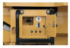
**ELECTRIC SERVICE CENTER.** A lockable compartment located just below the left side access platform contains key electrical components such as the remote jump-start receptacle, battery disconnect switch, circuit breakers and hood actuation switch. The maintenance free batteries are conveniently located under the electric service center.
