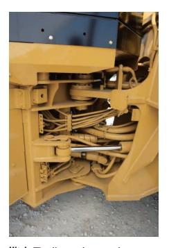
Hitch. The distance between the upper and lower hitch plates is an important contributor to machine performance and component life. The Caterpillar hitch design provides excellent load distribution and bearing life. Both the upper and lower hitch pins pivot on double tapered roller bearings — improving durability by distributing both vertical and horizontal loads over a larger surface area. The wide opening also provides excellent service access.
