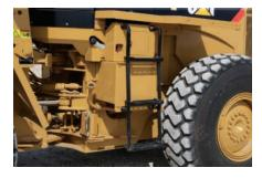
**ENTRY AND EXIT.** A ladder with aggressive tread pattern keeps debris build-up to a minimum. The ladder is at a 5° forward incline for easy entry and exit.
