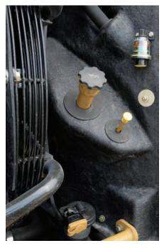
With the hood closed, quick checks of the engine oil level, coolant site gauge and air inlet indicator can be completed through the side service door. **ECOLOGY DRAINS.** Engine, transmission and hydraulic oils can be easily drained with standard-equipment ecology drains. An axle oil ecology drain is optional.
