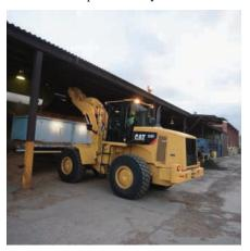
**LOAD SENSING HYDRAULICS.** The 938H features a load sensing hydraulic system that supplies flow and pressure for the implements only upon demand, and only in the amounts necessary to perform the needed work thus providing a more efficient loader.
